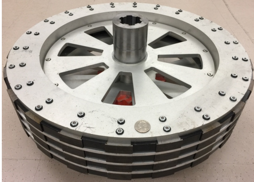
Fig. 4-25. Fully assembled inner rotor with three support rings.
