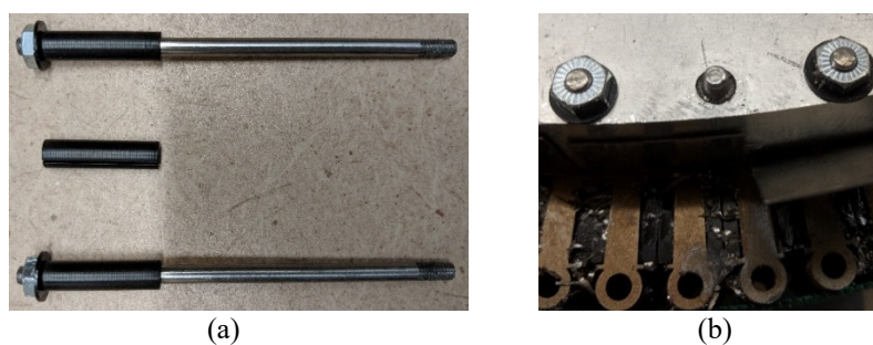
Fig. 4-84. (a) rods with plastic inserts and washers and (b) plastic inserts between the rod and the endplate.
