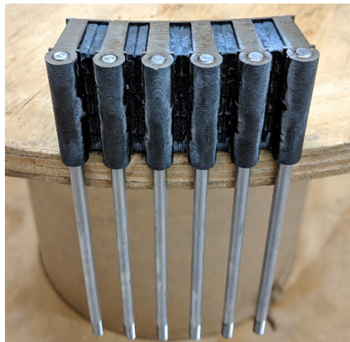
Fig. 4-86. Outer lamination with inserted magnets.
